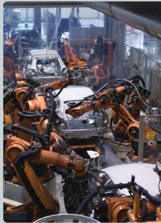
▲ Robotic arms carry out the assembly of cars on a production line
